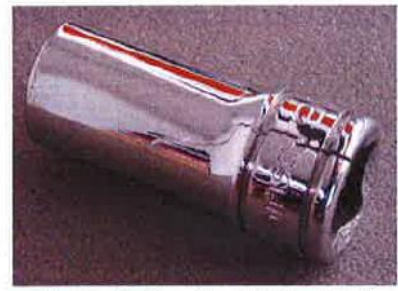
Photo 3: Crack at Drive End
