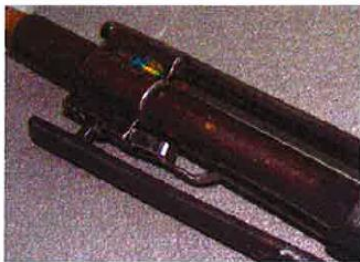
Photo 3: Worn or damaged locking mechanism.
