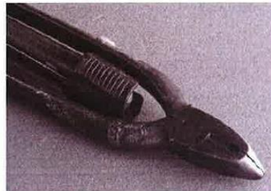
Photo 4: Worn vinyl or rubber casing.
