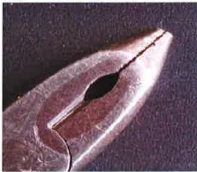
Photo 1: Wear & Tear at Jaw
