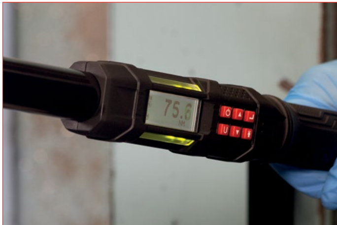
Dual progressive LEDs positioned both sides of the wrench provide an easy visual representation of torque progress
