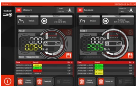
Displaying 2 transducer readings simultaneously
