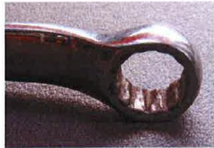
Photo 4: Worn-off Teeth (Wear & Tear)
